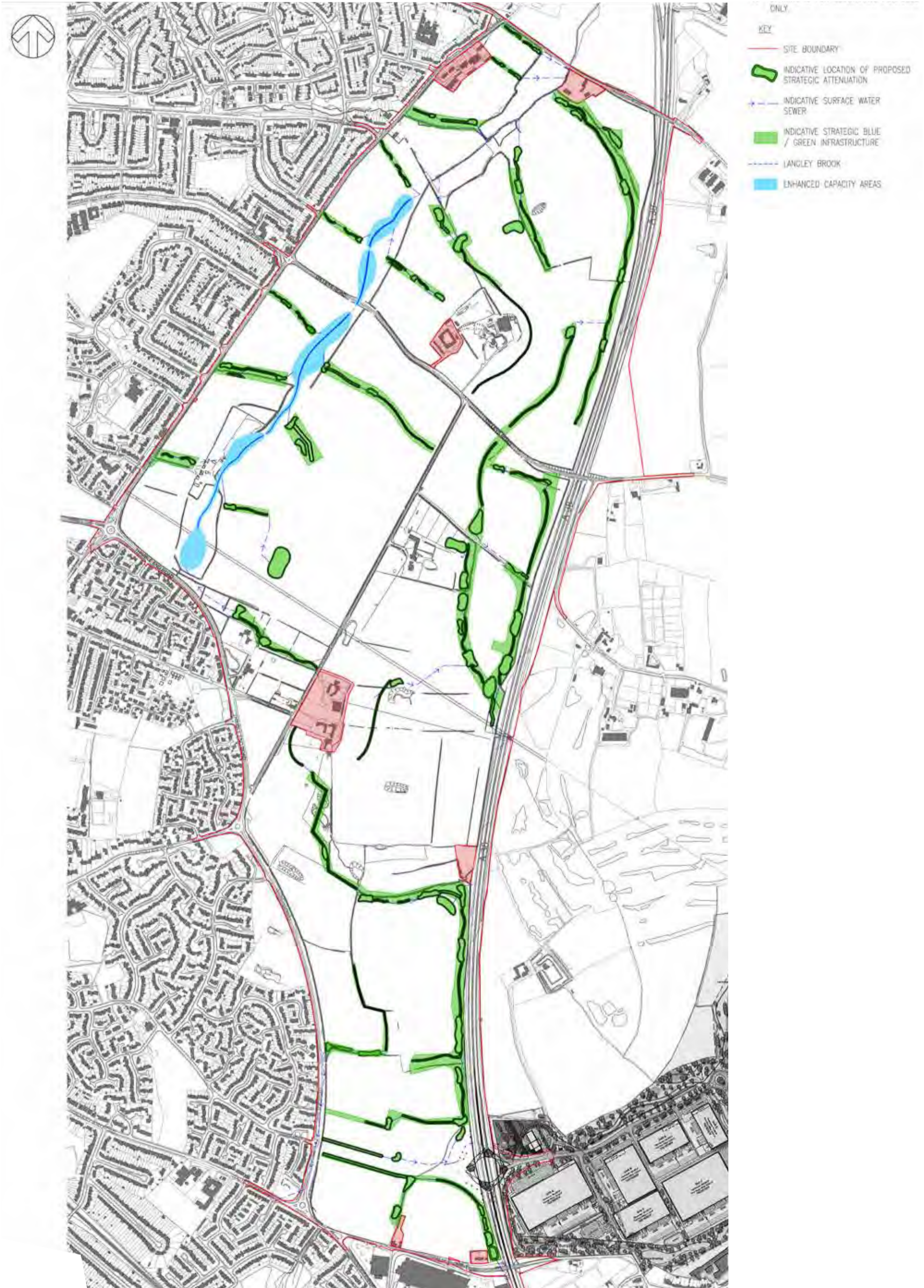
Figure 113. Strategic Surface Water Drainage Network
